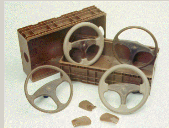
Injection moulded products from natural- fibre/plastic granules
